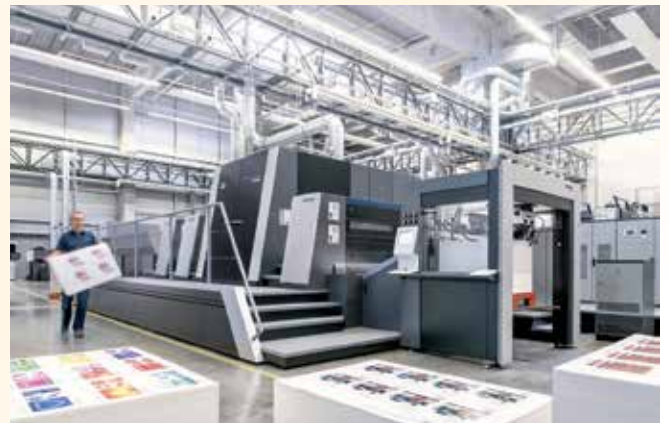
The Primefire 106 is the first industrial digital printing press for packaging in B1 format.
